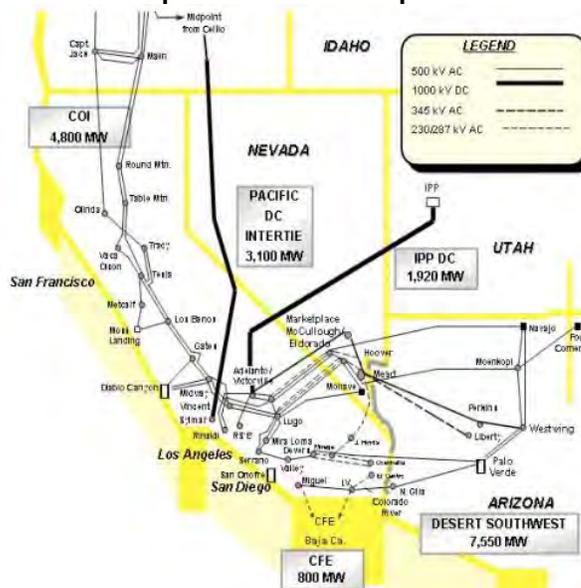
Figure 2 – California’s 18,170 MW of EHV Transmission Interconnections
